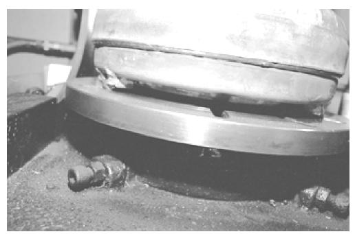
Clean, strong, and very consistent welds are made in the machine welder. Bad welds mean leaks and imbalance problems.
