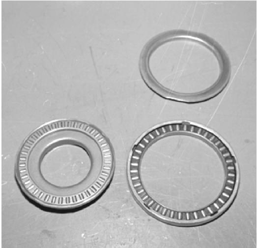
The large bearing (opened up for the picture) not only has more bearing rollers but more contact area to spread the contact energy across. Less friction and less heat buildup.
