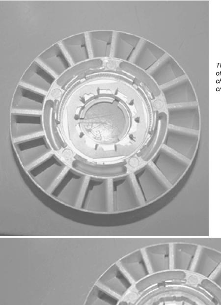
The cage sets in the bottom of the stator after the stator is checked for damage or cracks.
