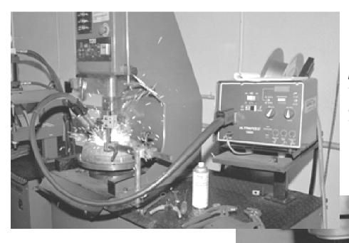
The entire jig is part of a welding rig. The turntable rotates and a perfect, consistent weld is made around the hub. This robot welding is far better than can be handdone.
