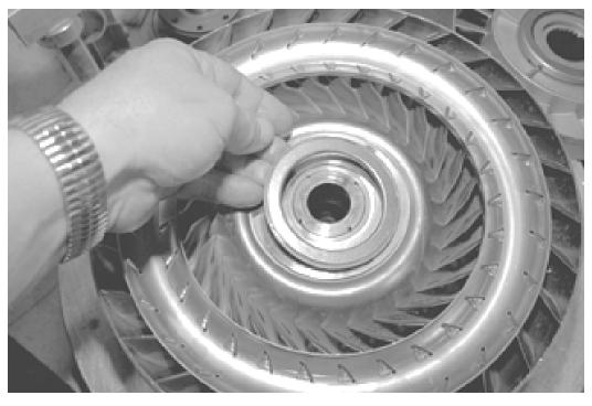
Speaking of conversions, there is a special hub made to replace the entire lockup clutch assembly to eliminate lock-up. This is sometimes used in off-road or very high performance units where the clutch is either not needed or has the potential to cycle too often or even outright fail do to extreme abuse. In almost every case, a street vehicle performs best with a properly functioning locking converter.
