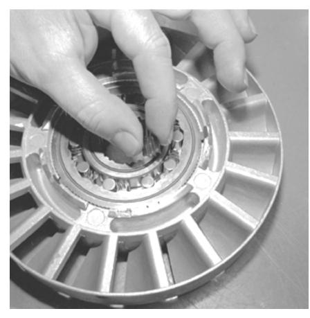
The accordion-like Sprag springs keep the rollers pressed to one side until the rollers and cam are engaged and return the rollers. Broken, damaged, or compressed springs won't do.
