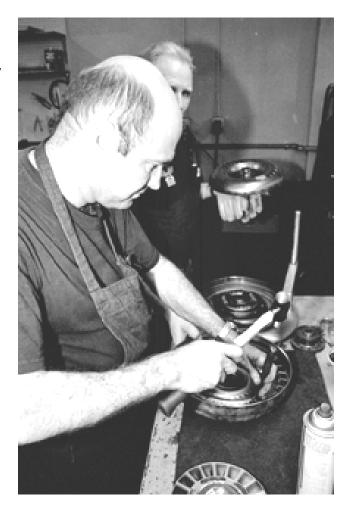
In addition to altering blade angle as required, William deftly uses a punch and hammer to tighten every fin prior to welding. More important small details.
