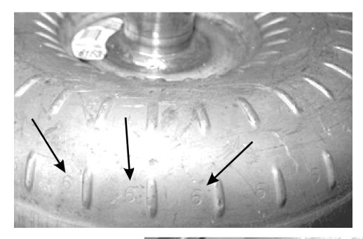
The stamped numbers in many converters tell you details about stall speed and impellers. See sidebar #1
