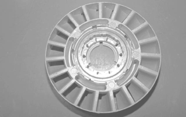
The Sprag cam sets over the top of the cage to retain it. The cam must be in perfect shape or it will rapidly fail.
