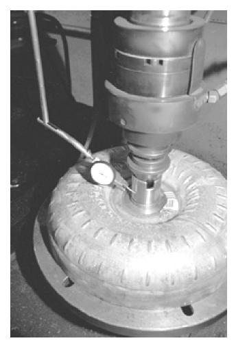
The new hardened hub sets on the converter housing in a special jig. The housing rests flat and the conical fitting locates the hub in the dead center.
