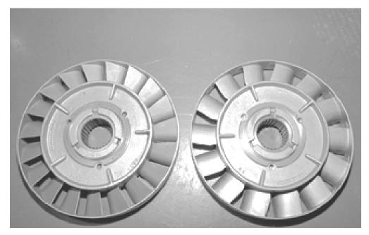
The stator on the Right is the rare high-stall part used in a very few 4.3 liter S-10's and turbo cars but never in the Corvette or Camaros
