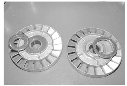
The stator on the right is the latestyle part with the large one-piece enclosed Torrington bearing. The other is the early style with the small Torrington with separate staked-in race. The right choice is obvious.
