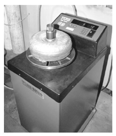
parts swapped for others and welded back together. Some get new parts but they are of poor quality. A vast majority are not well balanced or are out of spec. When converters fail, they throw debris throughout the trans and pretty well thrash the works.
