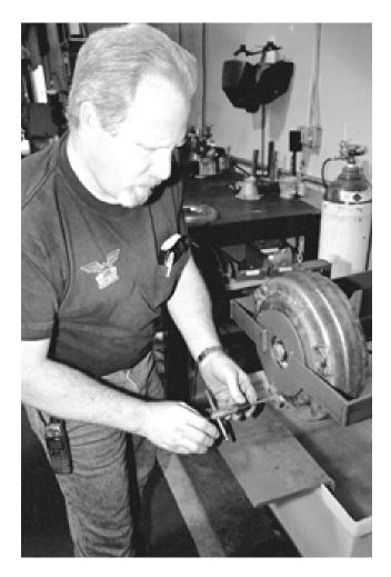
Even details like the threads in the mount lugs are checked and cleaned. Shops that do this kind of quality rarely see failed returns because they pay attention to details. How many times do you want to replace a converter?
