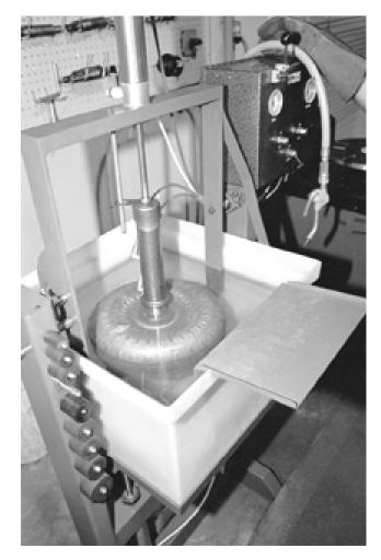
All converters are pressure-tested at 120 psi. Not even the smallest leak is acceptable.
