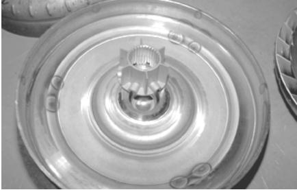
If you want to eliminate the lock-up, the entire clutch assembly can be replaced with this machined hub/ spacer.
