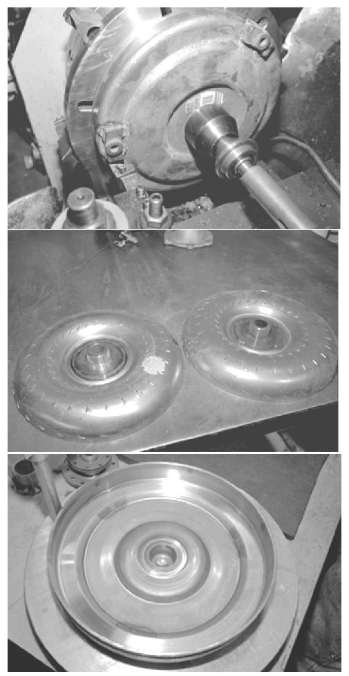
The front half is flipped over and the mounting lugs are trued. You'd be surprised to find how many of these are crooked, beat up, or stripped.
