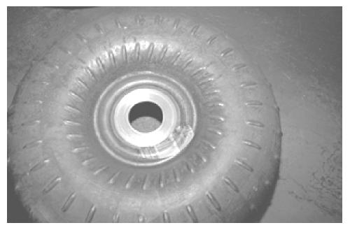
A damaged hub. Rather than try to repair or re-cut the hub, Phoenix will remove it and replace it with a new hardened hub.
