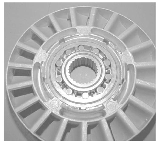
You can see how the rollers fit into the cam. They require correct clearances so any wear is a death warrant.
