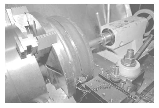
The converter is cut apart in a lathe which cuts away the weld holding the halves together. William has just the right touch to pop the converter apart without beating it up. The hammer splits any remaining weld material.
