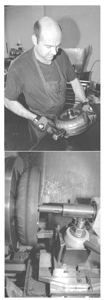
The front half is also turned to clean weld debris and deepen the shelf cut so the halves can be assembled at the correct height later.
