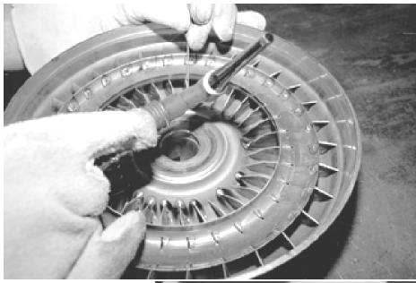
Each and every fin is spot-welded with a TIG machine by hand. Greg says it's important not only to weld each one, but make sure each weld is exactly the same and holds well. It takes skill and practice.
