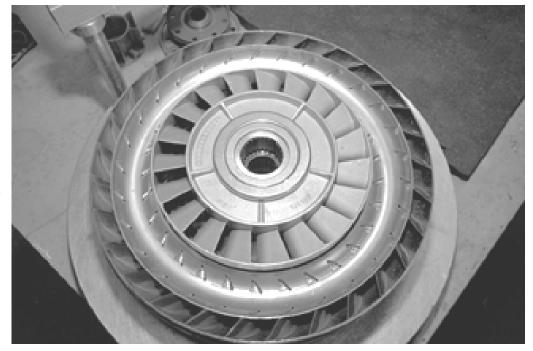
This is the complete internal assembly with the stator on top - ready to cover.
