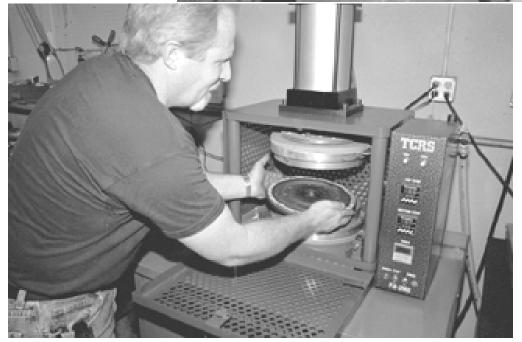
No, Greg isn't making lunch - he's setting a clutch in the bonding oven. The Kevlar clutch material is glued to the plate, making sure it is centered and in it goes.
