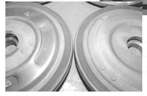
On the right is the woven carbon fiber clutch used in 1998 and later severe duty units. On the left is the carbon composite clutch which is a durable and heatresistant material used in most applications 1992-98.
