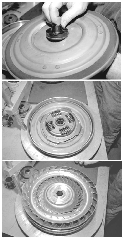
This phenolic insert sets end-play and seals the input shaft to the clutch hub as well as determines overall converter height. They come in various sizes for adjustments.
