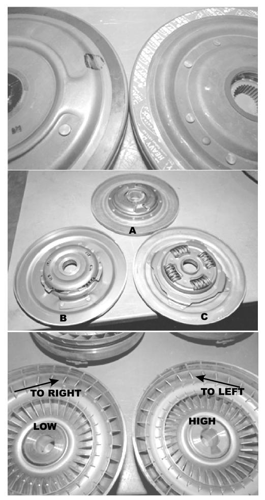
On the left is a paper faced clutch which is only good for the lightest-duty applications and which Phoenix never uses in its converters. On the right is the Kevlar material Greg bonds to upgrade or replace worn facings.
