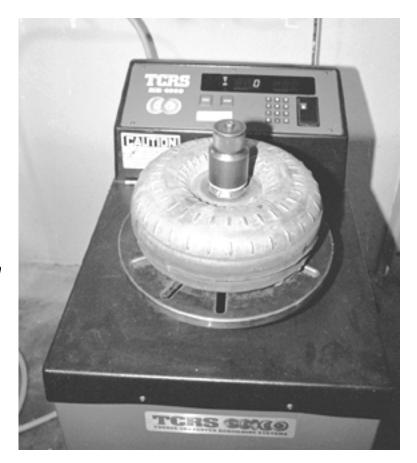
That zero on the balancer readout means just what it says. Zero balance is not an option if you want a smooth and durable converter.
