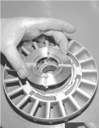
An aluminum spacer is installed instead of the phenolic spacer for high performance or severe use.
